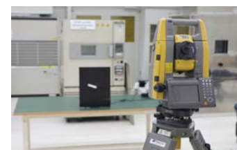
Auto-tracking durability test against rotating object.
