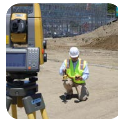
Auto-tracking test under high speed vibration conditions
